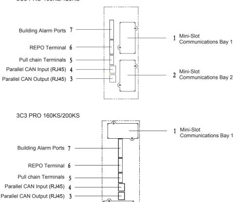
1 (2). Expansion slots: Slots exclusively available on the 20KS-200KS models and only accessible by users with special requirements. Standard users have no access to the slots.
