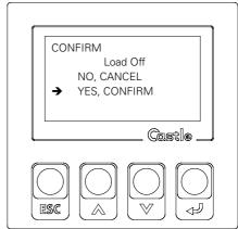
The 3C3 PRO series can start and operate with battery in the absence of AC mains supply, with a panel display similar to that in the case of AC supply. You can just follow the instructions displayed on the panel to start or shut down the UPS with battery:
